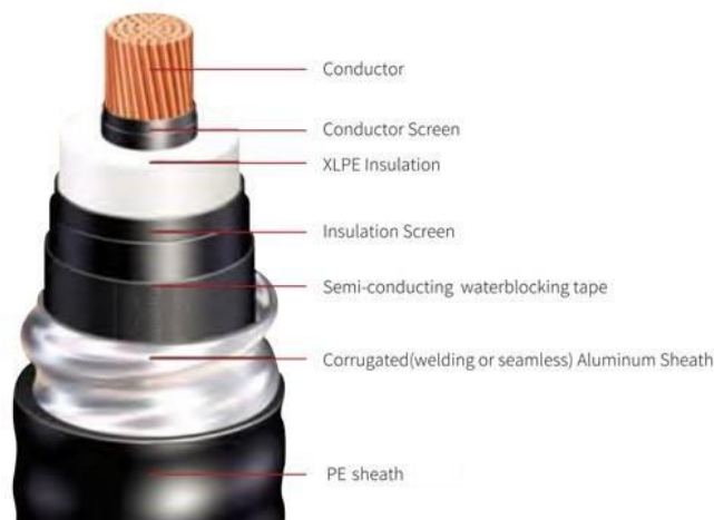
Figure 3 Single-core cable with corrugated aluminium sheath earth screen
